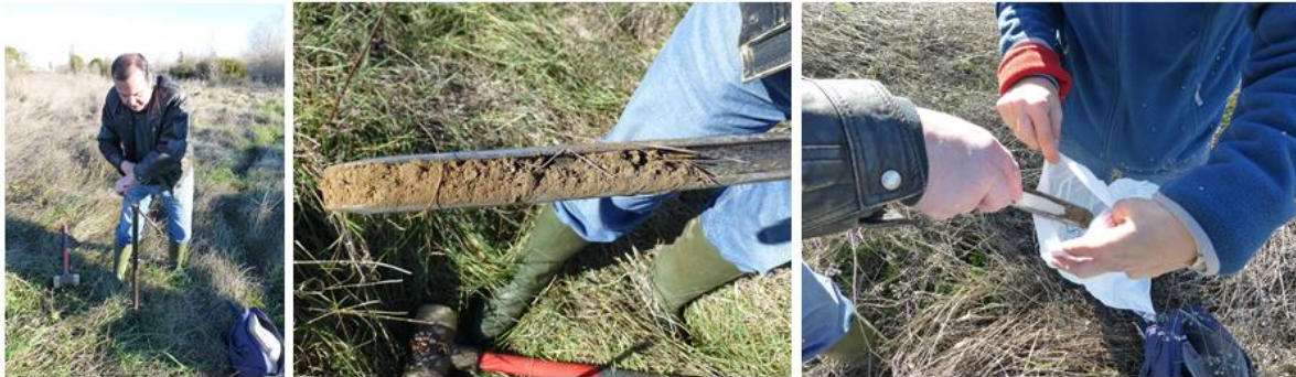
Figure 6: Soil sampling using an auger, collecting the top soil (0 -15 cm)
