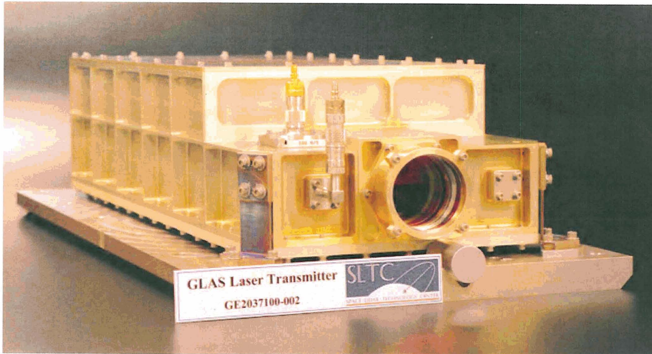
Figure 2. External photograph of the GLAS laser serial number 2. Visible is the output port of the laser beam, the mounting flexures, quick disconnects (remove before flight) for venting and purging with air, and a reference mirror used to align the pointing of the laser beam mounting feet.
