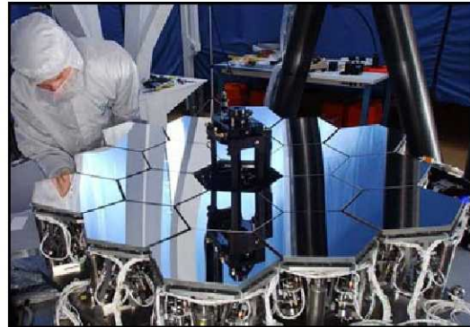
Figure 9: Fully functional 1/6 scale telescope model used to develop wavefront sensing and control process and algorithms
