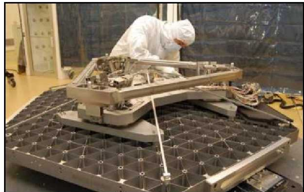
Figure 8: A primary mirror segment entering cryogenic testing (left), mechanized segment mount assembly provides 6 DOF and radius of curvature adjustment (right)
