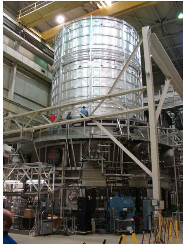
Figure II-2. SES GHe Shroud in -03 (OTE GSE) Test Configuration
