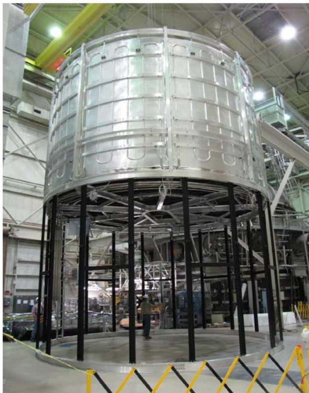
Figure II-1. SES GHe Shroud in -01 (ISIM) Test Configuration
