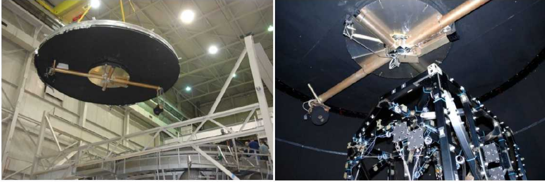
Figure II-7. PG Camera and Boom Assembly Mounted to Helium Shroud Ceiling
