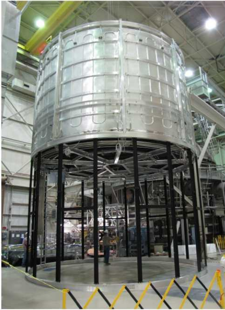
Figure II-2. SES GHe Shroud in -01 (ISIM) Test Configuration
