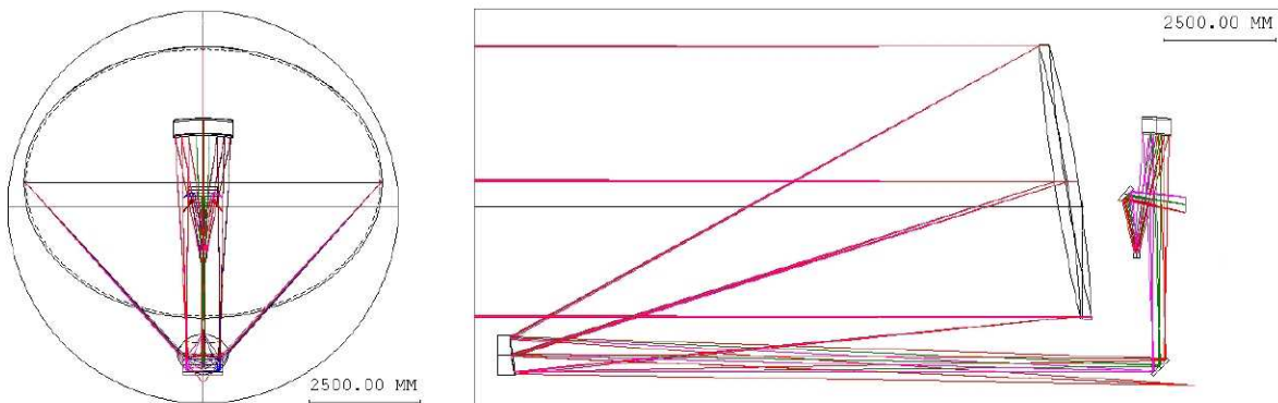
Figure 13a/b. Off-Axis 6x8 meter TMA shown in a 30-foot diameter shroud.
