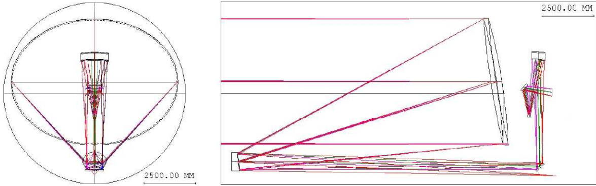
Figure 13. Off-Axis 6x8 meter TMA shown in a 30-foot diameter shroud.
