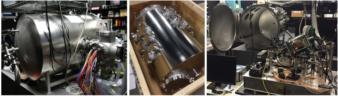
Figure 6. Left : the VNT chamber as used in TDEM-10 (MS#2). Center : the modified chamber received on 9/20/16. Right : the upgraded VNT chamber following successful testing on 9/21/16 with a combination of port blanks and previously tested feedthroughs, ready to be used toward meeting TDEM-13 Milestones #1.5, #2.5, and #3.
