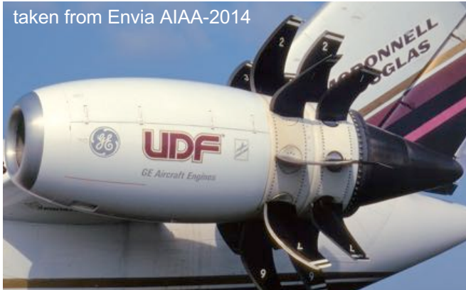
GE36-UDF propfan demonstrator engine installed on MD-81 test bed aircraft (8x8)
