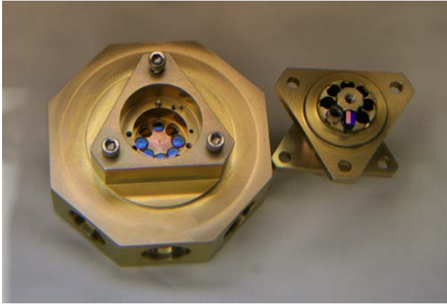
Figure 5. The central prism assembly (left) and field lens assembly (right) of the MASTAR instrument. Both assemblies are shown inverted relative to their final orientation in the integrated instrument. Reimaging optics for each of the 8 apertures are visible as small circles in the center of each component.
