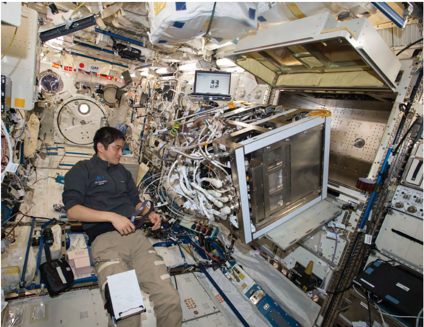
ISS crewmember Takuya Onishi functional-checking the Electrostatic Levitation Furnace (ELF) facility (ISS049E002367).
