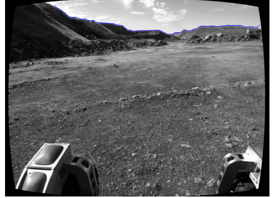
Fig. 5. Example of horizon curve (blue) detection over a rectified image taken by on-board camera.
