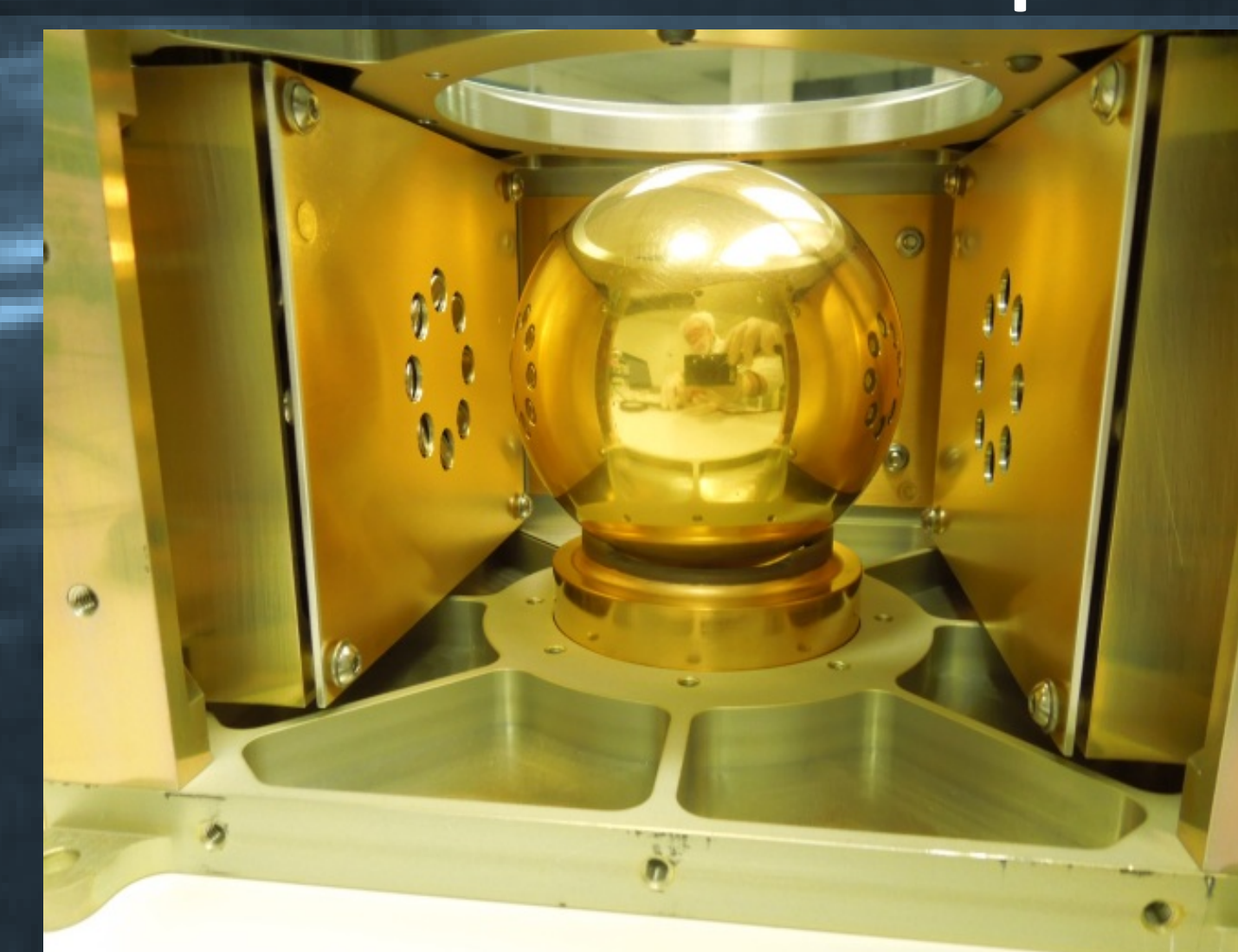
Figure 4. Interior of UV-LED, showing gold-coated proof mass and 2UV-LED boxes on either side
