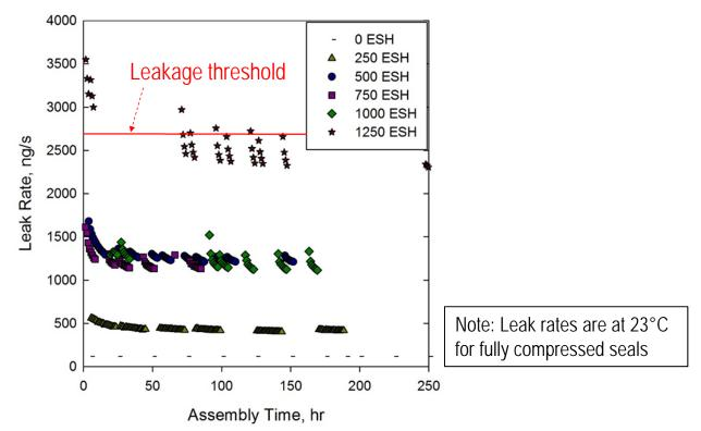
Leak rates for baseline seals also decreased as tests progressed, although magnitude of decrease was less than what was seen for seals with TiO<sub>2</sub> additive
