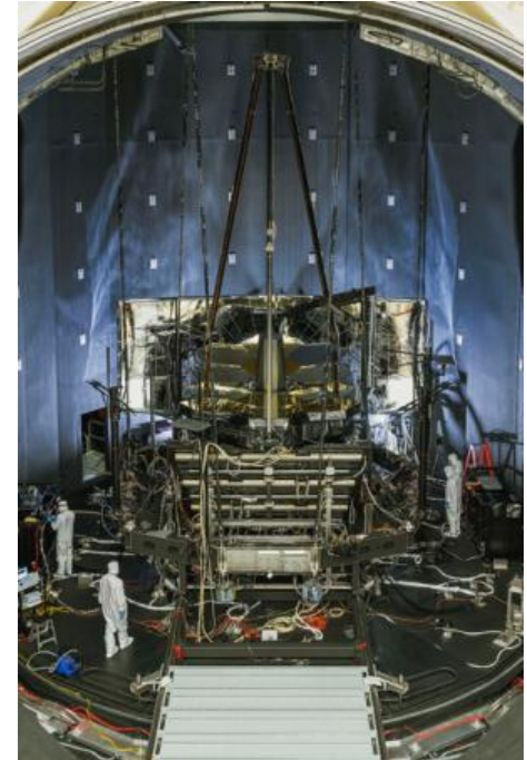
Thermal Pathfinder: Verified all thermal environment/boundary conditions (e.g., sunshield layer 5 thermal simulator, ISIM radiator sinks)
