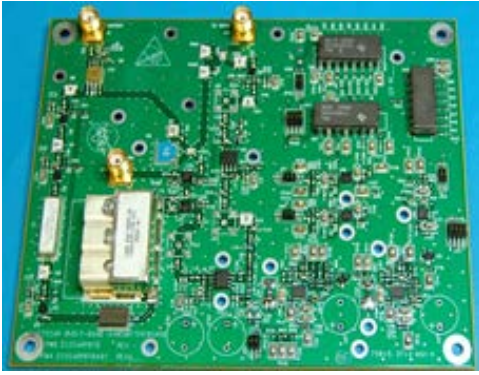
Figure 4 SESAR's compact and highly efficient Radar Transceiver Modules are distributed over the antenna panels driving each of the antenna elements.
