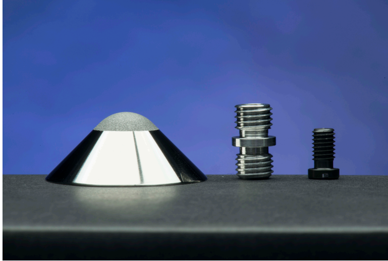
Figure 14. Sphere-cone model, aluminum rear stud and Vespel insert.
