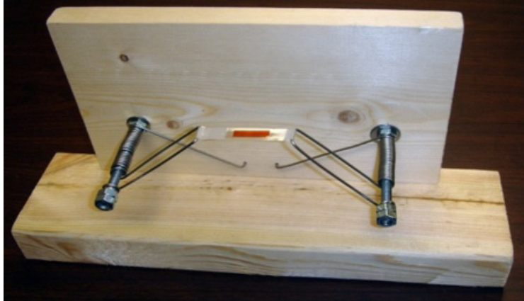
Figure 7. The bend-test mechanism in its idle state; the polymer being tested rests atop the Kapton stretched across the center, with the space exposed surface face down.
