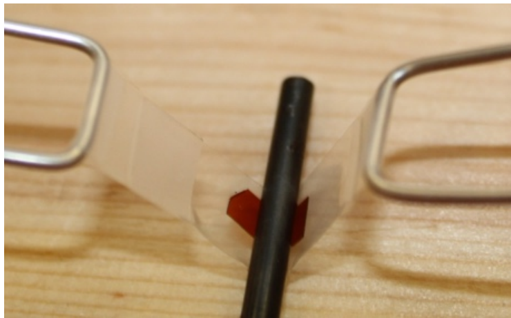
Figure 8. The bend-test mechanism in its testing state; the polymer being tested wraps around the circumference of the mandrel with the space exposed surface in tension.
