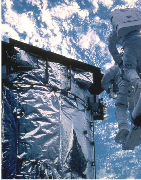
Figure 1. Example of cracking of the aluminized-Teflon FEP insulation on the HST after 5.8 years of space exposure (Ref. 2).
