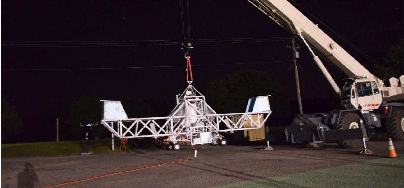
Figure 6: In both Fort Sumner and in Palestine, system-level tests of the payload were carried out both in the high bay facility and outside using a mobile crane.
