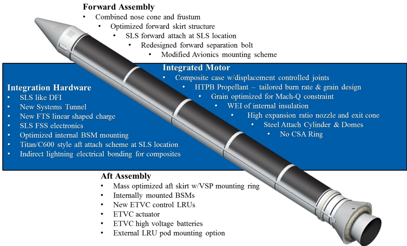
Figure 3. BOLE Design Changes Overview
