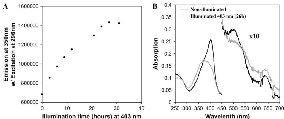
**FIGURE 7** (A) Effect of 403-nm illumination time (heme excitation) on the protein's fluorescence emission intensity at 350 nm obtained upon 296-nm excitation. Fluorescence emission spectra were acquired after 0, 3, 6, 9, 12, 21, 24, 27, and 31 h of illumination at 403 nm. (B) Absorption spectra of native HRP A2 (solid line) and of HRP A2 illuminated for 26 h at 403 nm (shaded line).
