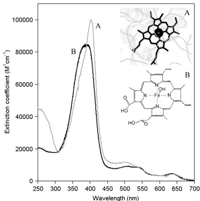
FIGURE 2 Absorption spectra of hematin (*solid curve*) and native HRP A2 (*shaded curve*). Insets show the heme group in peroxidase (A) and the hematin molecule (B). The hematin extinction coefficients were taken from Du et al. (32). In native HRP A2 the absorption below 300 nm is mainly due to aromatic amino acids and cystines. The peaks around 403 nm and above 475 nm are only due to heme absorption.
