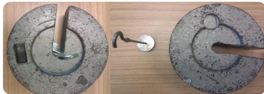
Figure 2-21: 5 Kg Weight and 0.05 Kg stand
