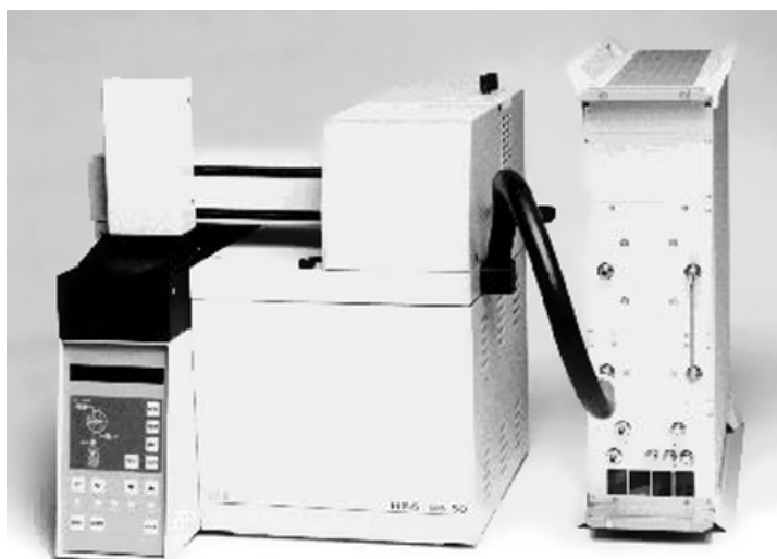
Figure 1. E-nose system used as a stationary device (photograph by courtesy of Udo Weimar).
