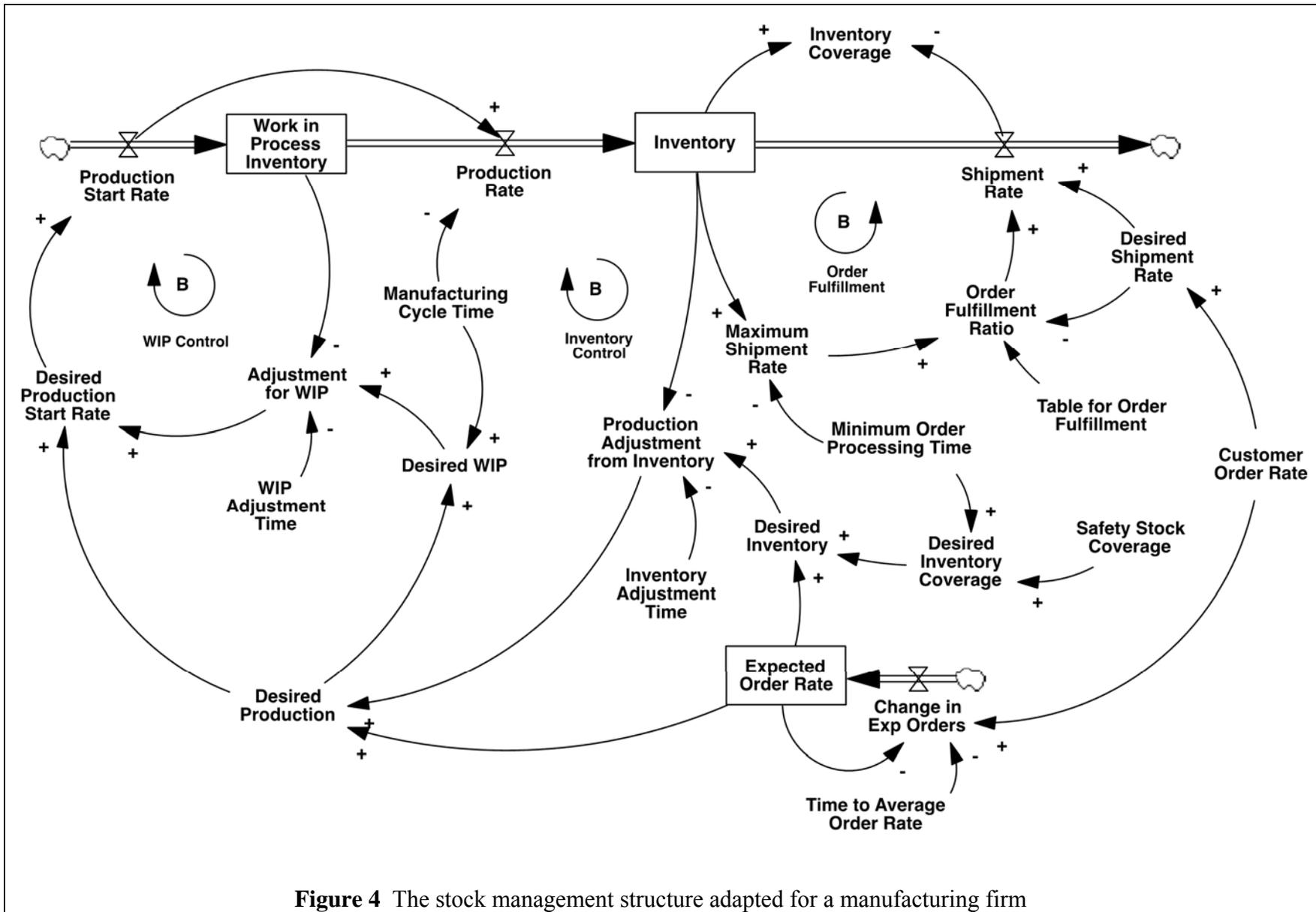
**Figure 4** The stock management structure adapted for a manufacturing firm
