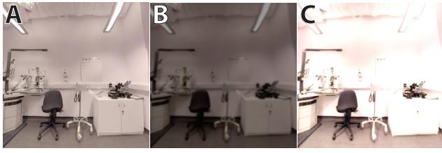
Figure 2: Disability Glare. (A) The source image; (B) a blurred and contrast-gain modulated duplicate of the source; (C) Output image, computed by summing together (A) and (B).
