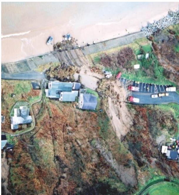
Fig. 10 Landslide at Nefyn. Note the dark mudslide at the top of the slope (right hand side of the image) that could have triggered a similar debris flow above a residential property. Image courtesy of North Wales Police
