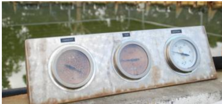
Figure 3.3 A Dial thermometer on top of the concrete wall
