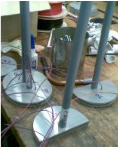
Figure 4.19 Semi-circular diffuser attached to inlet and outlet of hot brine
