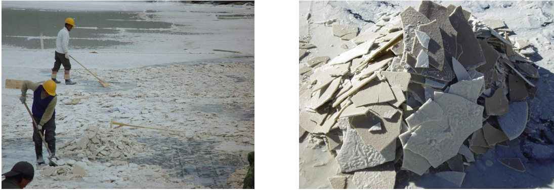
Figure 2.11 Workers collecting lithium carbonate (left) and the harvested lithium carbonate (right) at the Zabuya salt lake in Tibet
