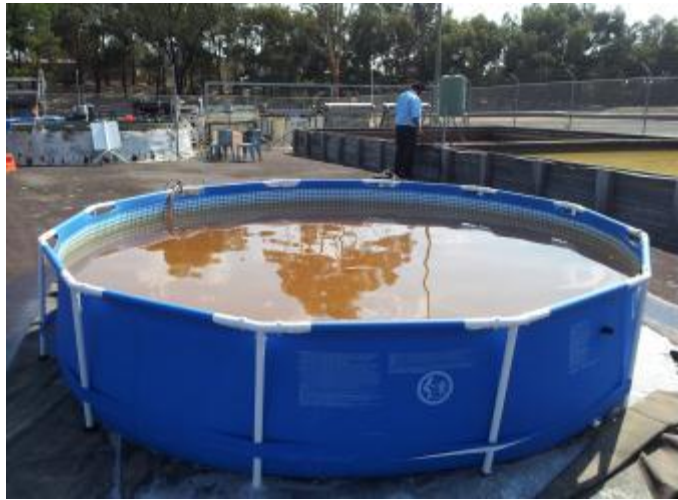
Figure 3.16 A Circular portable pool used as a storage pond.
