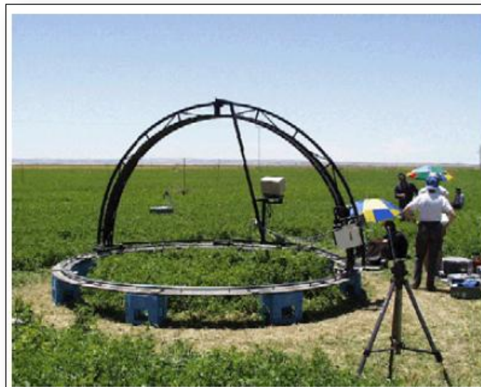
Figure 2.12 (Schaepman, 2006) shows a goniometer used in the field.
