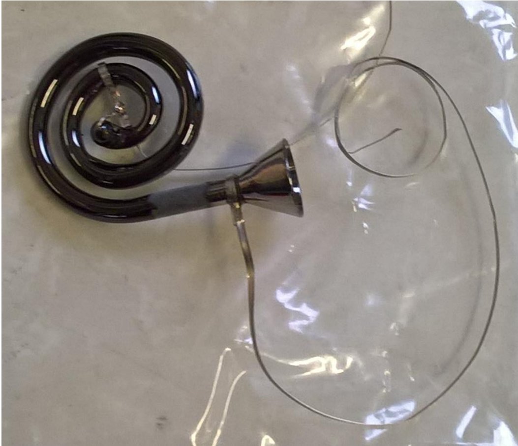
Figure 2.8 – A photograph of a single channel electron multiplier. Clearly visible is the continuous-dynode spiral structure, as are the electrical connections for providing the bias across the multiplier.
