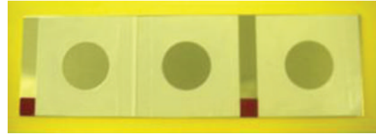
FIGURE 2: Image of the active sample including the maskholes and coating free areas used in the cathodic breakdown test.
