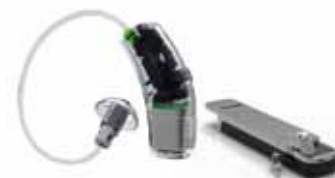
The hearing aid powered by a direct methanol fuel cell - to be further developed by Fuel Scale Integrate.
