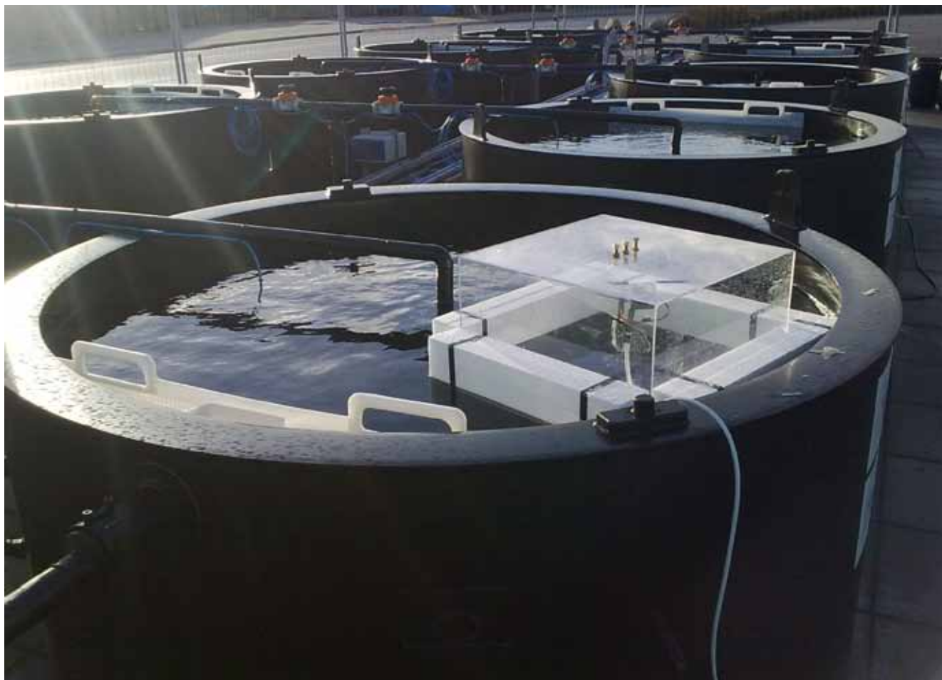
Large cultivation ponds at AlgaeCenter Denmark. The floating incubation chamber is placed in a cultivation pond containing natural seawater and Sea lettuce. Transparent chamber enabled solar light energy to the photosynthesis of the algae. Vigorous air bubbling ensured biomass mixing.
