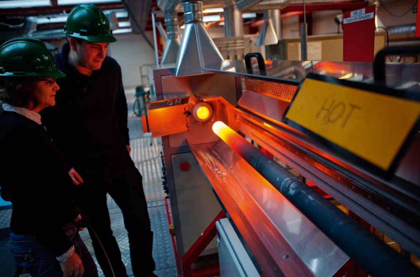
A new lab-scale rotary kiln simulator has been designed and constructed to study clinker formation mechanisms and kinetics. (Photo: Klaus Holsting)
