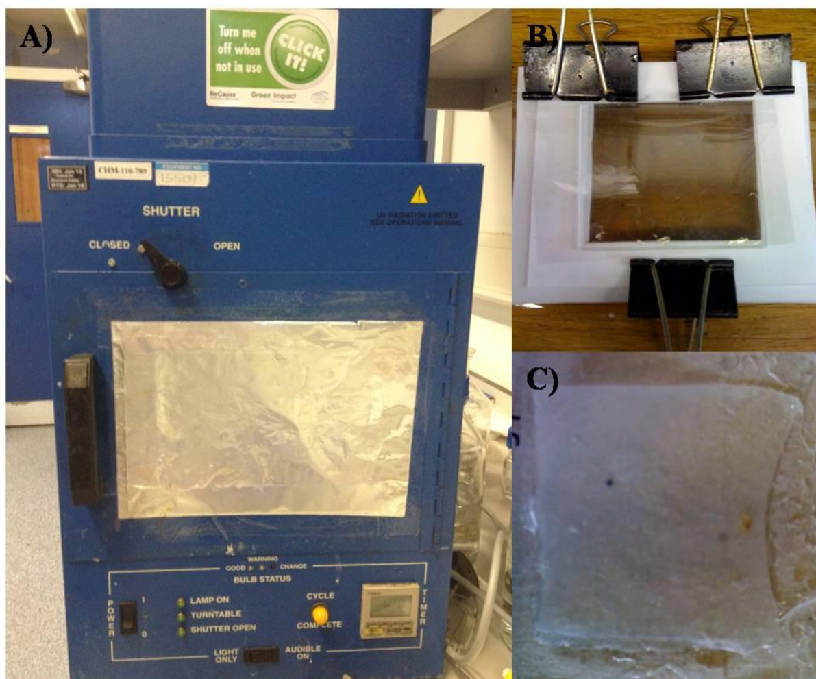
Figure 2.6 Experimental set up for the polymerisation of semi-IPN and graph conetwork (A) Dymax UV curing system, (B) mould for polymerisation and (C) example of the polymerised hydrogel.
