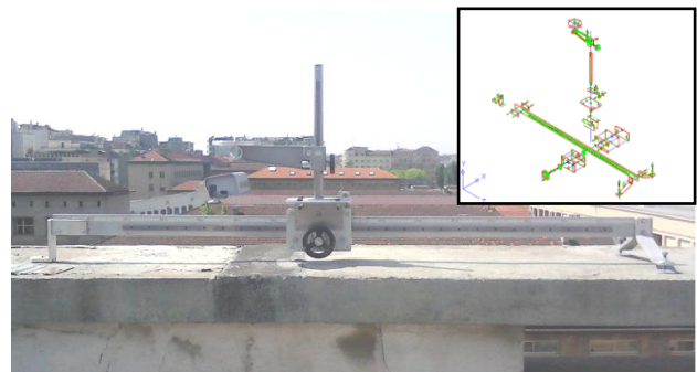
Figure 12. Micrometric slide for controlled deformations
