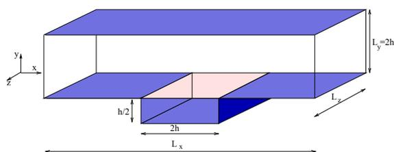
**Figure 1.** Fig.1 Scheme of the channel-cavity domain. Dimensions are defined with reference to the half channel height,  $h$ . The cavity is located at the centre of the lower wall. The size of the computational domain is  $L_x/h = 4\pi h$  and  $L_z/h = \pi$ .
