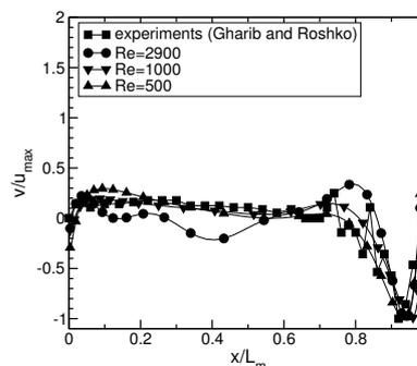
**Figure 4.** The  $v$  velocity in the  $y$  direction, divided by the maximum of the streamwise velocity component, versus the distance from the edge of the cavity. The velocity profiles obtained for different Reynolds number are compared with the laboratory results by Gharib and Roshko (1987) [1], obtained for a cavity placed along a boundary layer in cylindrical symmetry (Reynolds number equal to 24000).
