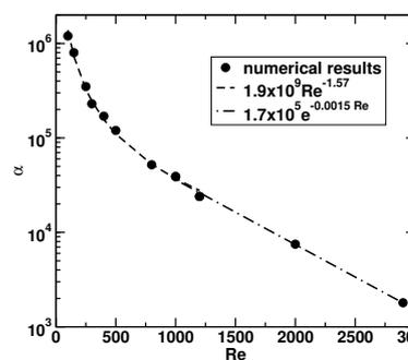
**Figure 2.** The ratio  $\alpha = \frac{\langle pv \rangle}{\langle E_v \rangle}$  between pressure and kinetic energy flow across the cavity mouth, versus  $Re$ . The value of  $\alpha$  initially falls down with  $Re^{-1.57}$ , then above  $Re \simeq 1000$ ,  $\alpha$  sets to an exponential asymptote.
