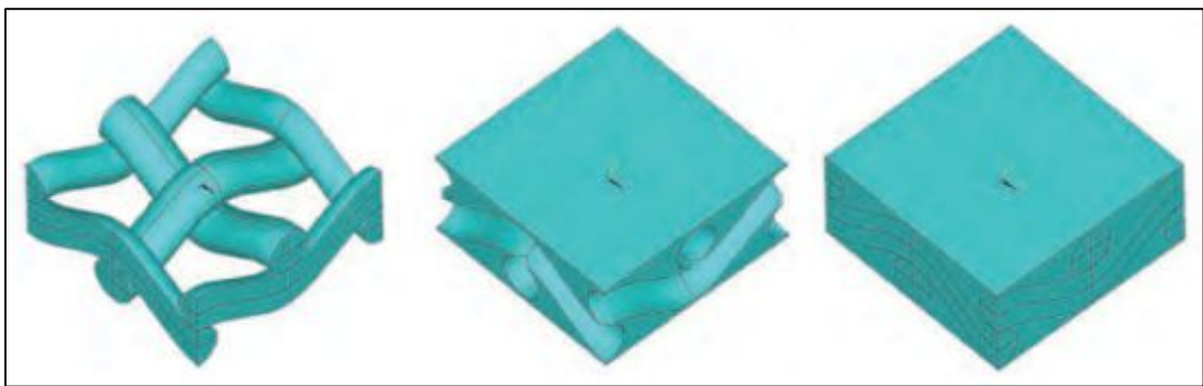
Figure 1.1: Geometrical model of composite woven structure (woven reinforcement, matrix, composite) (Whitcomb, J. and Srirengan, K, 1996)
