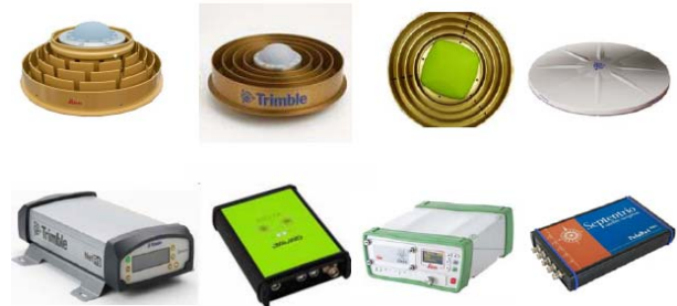
Figure 2. Commonly employed antennas (top) and receivers (bottom) within the MGEX network
