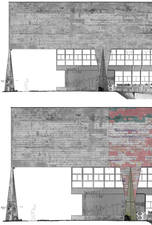
Figure 6. Data representation of a sample of elevation; above, view of the CAD two-dimensional representation superimposed to the DEM; below, example of degradation characterization
