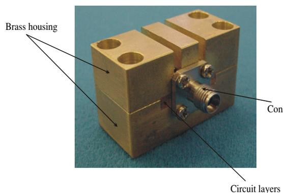
**Figure 9.** Photograph of a complete layered coaxial device.
