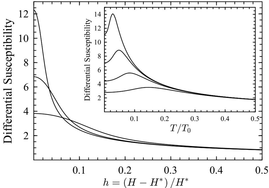
**Fig. 5.** Differential susceptibility,  $\chi_0^{-1}(\partial m/\partial h)$ , as a function of applied field  $H$  at temperatures  $T/T_0 = 0.05, 0.1, 0.2$ , for a two dimensional metamagnetic critical point. Inset: Dependence of  $\chi_0^{-1}(\partial m/\partial h)$  on temperature  $T$  at  $h = .01, .02, .04, .08$ . (Normalizations discussed in text.)
