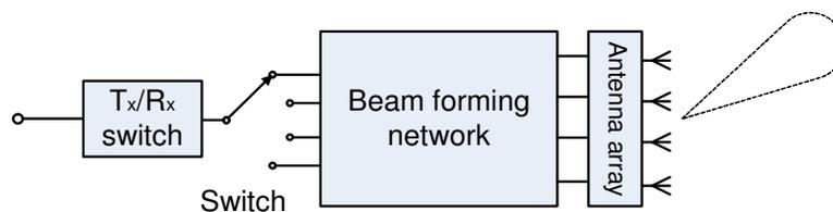
Fig. 1. A transceiver system with switched beam-forming capability.
