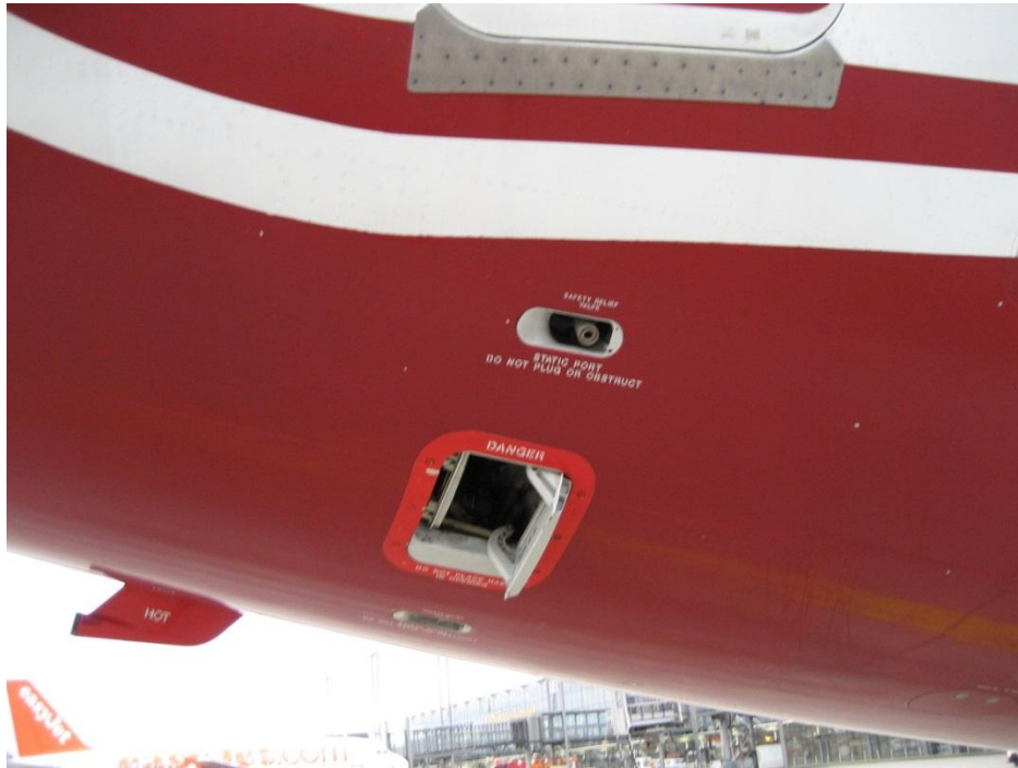
Figure 7.3 Boeing 737-800: outflow and relief valve
