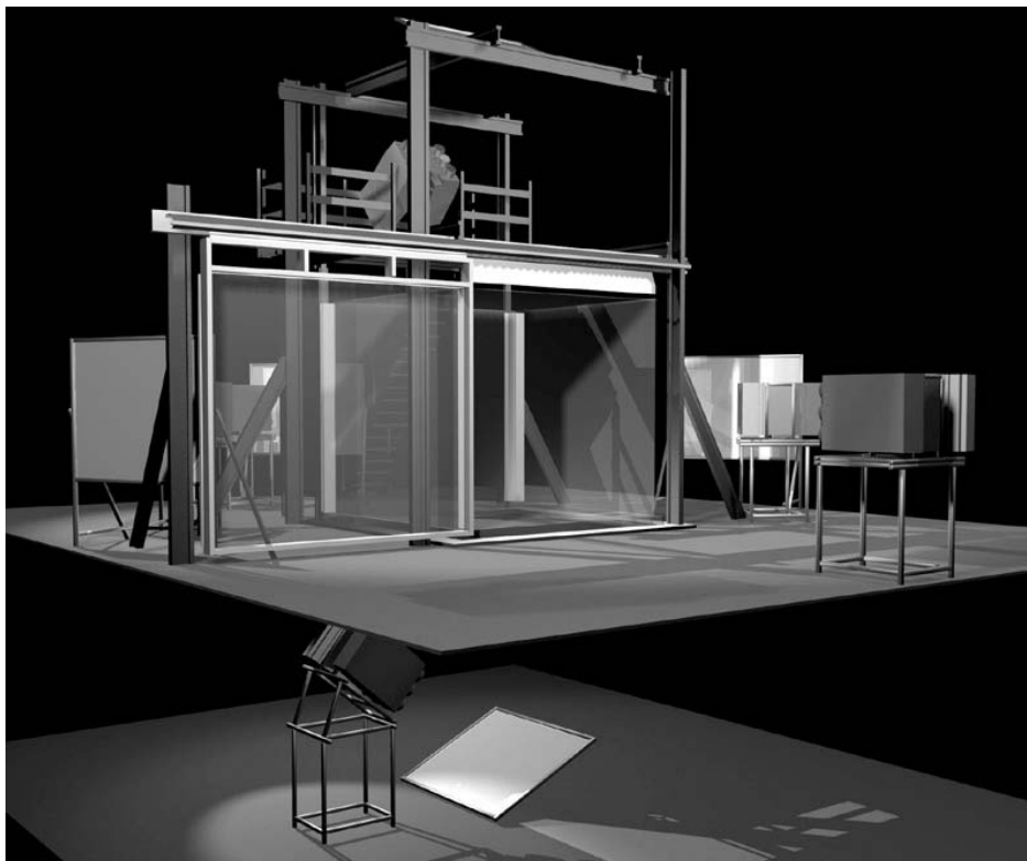
An impression of a 6-walled I-space virtual reality system (image courtesy of Barco N.V.). The I-space installed at the Erasmus is a 4-walled system, without ceiling and sliding back wall.
