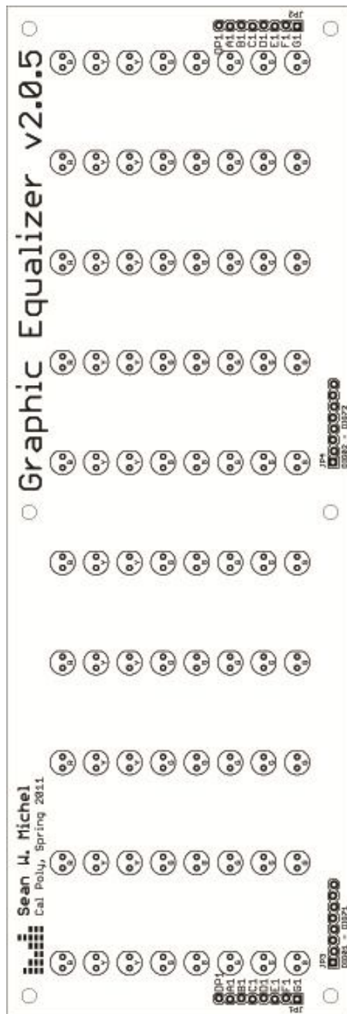
Figure 13: Display PCB Component Locations. Each LED has a ring with a "clipped" edge that represents the cathode. Color identifiers are covered by the component itself.
