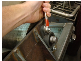
Figure 10. Adjustment of bearing
