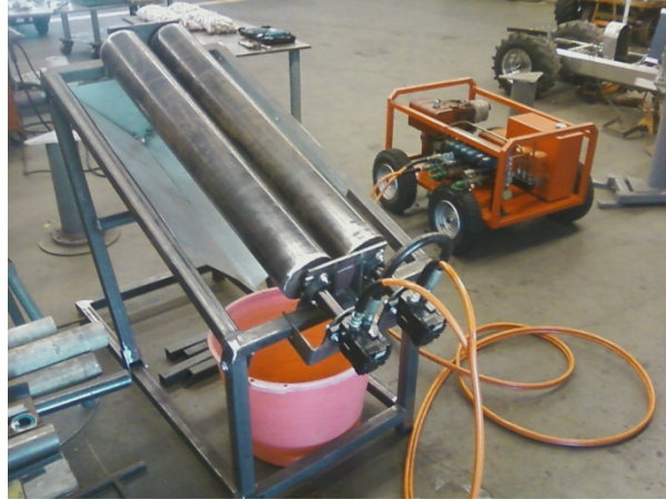
Figure12. Walnut cracker completed and connected to power supply
