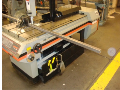
Figure 9. Cutting of main frame member using marvel 8 band saw
