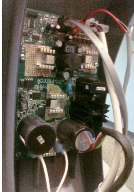
Figure 11 Precor PCB Board, one function is to convert from AC to DC
