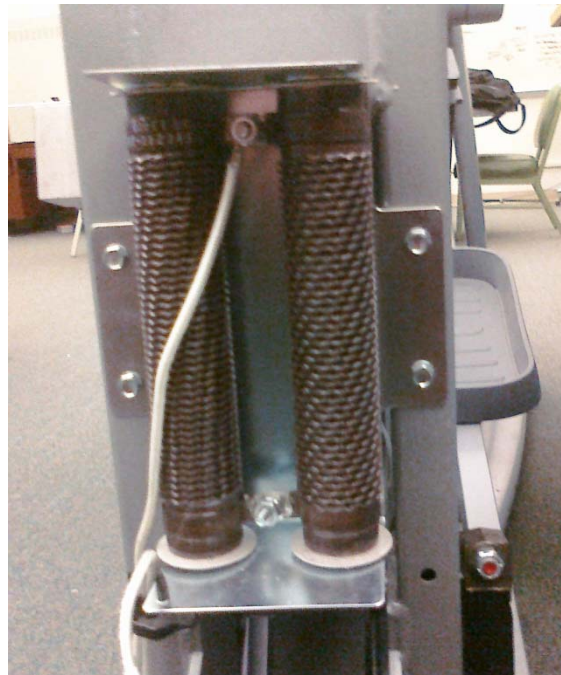
Figure 12 Elliptical Load Resistors, Two Parallel 20 Ohm Resistors
