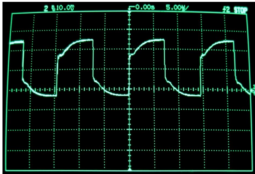
Figure 5-7: Emitter Current, 2A/div, 5µs/div, 50% load
