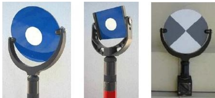
Figure 3.4: Different types of target used for 3D model registration
