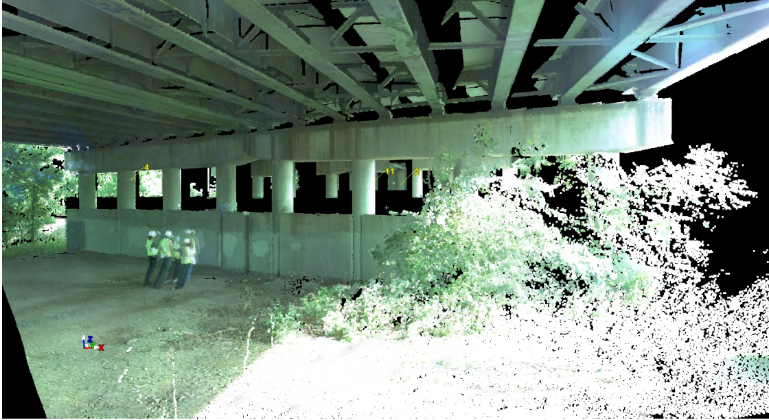
Figure 3.6: A registered 3D model of point clouds acquired from Cyclone
