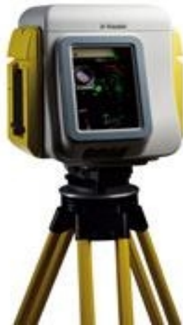
Figure 2.2: A sample for 1 laser scanner with panoramic view (Mensi Trimble)
