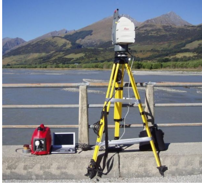
Figure 1.4: Leica Scanstation 2 terrestrial laser scanner (slcassociates.co.uk)
