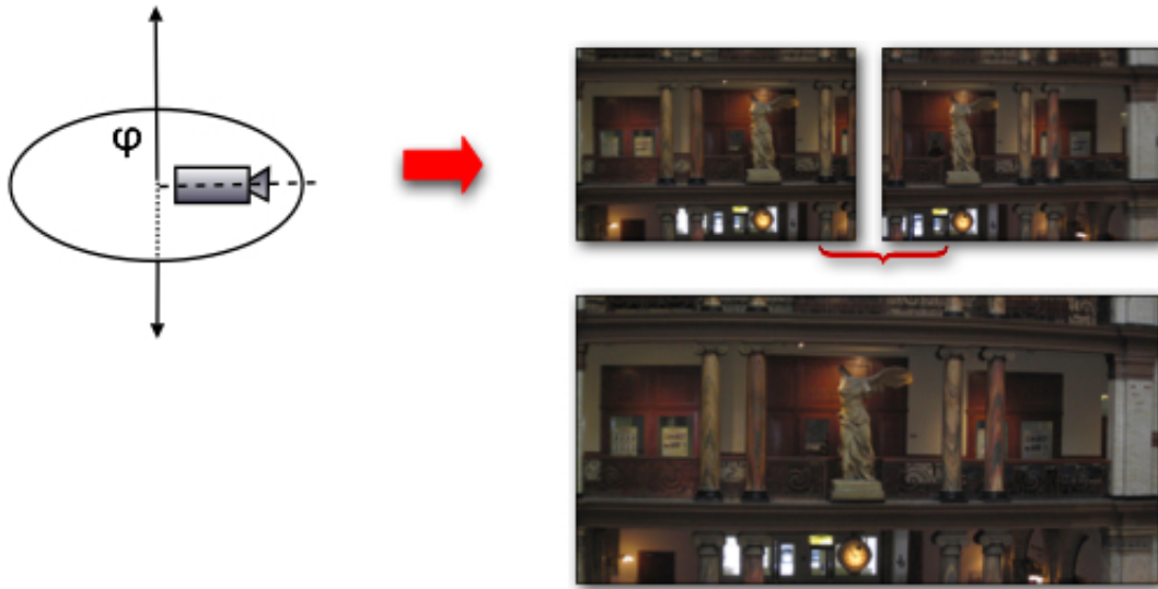
Figure 1.9: Image Mosaicing. Blending of two images to create a new image with a wider Field of View
