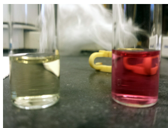
Figure 2.13. (Left) 0.5 mM Sp 2 in MeOH (Right) 0.5 mM Sp 2 in MeOH upon addition of 100 \mu L of pyridine.
