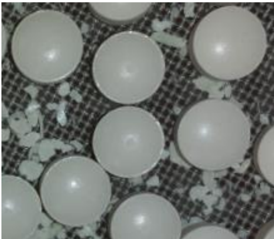
Figure 28 – Reclaimed material from the 21% X-B1 formulation was sieved using a sieve with a 600 \mu m opening (30 mesh). Compacted plate-shaped fragments are observed in the reclaimed powder.
